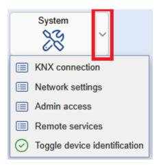
When *Toggle device identification* is clicked, LED2 starts blinking red and green. Click it again to stop this process.
